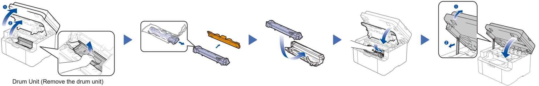
Drum Unit (Remove the drum unit)
