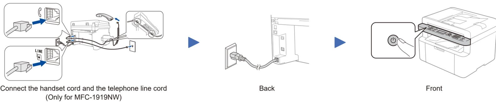
Connect the handset cord and the telephone line cord (Only for MFC-1919NW)
